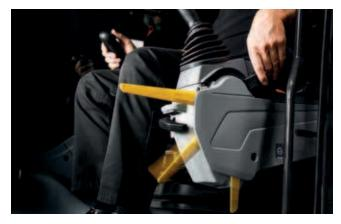
The pilot shutoff lever offers enhanced safety in the cab.
