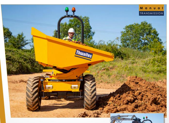
The Thwaites 3 Tonne Power Swivel, Stage V dumper is manufactured with contractors and hirers in mind – ensuring operator safety, reducing risk on site and improving performance. Powered by an 18.1 kW 3-cylinder Yanmar engine, delivering 107 Nm max torque for optimum traction and control. This machine is driven by a Manual transmission.
