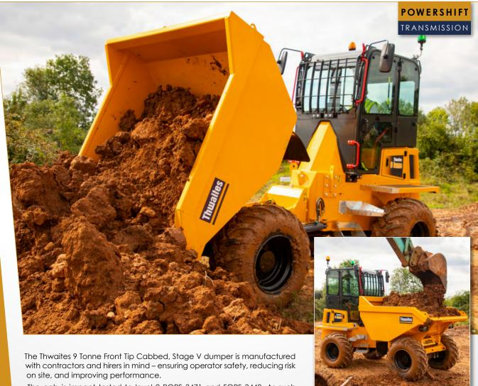
The cab is impact tested to level 2 ROPS 3471 and FOPS 3449. As such all Thwaites cabbed dumpers are approved for use by the UK Major Contractors Group. Front Tip dumpers allow the machine to be easily and safely loaded, with a straightforward tipping action that places the full bucket of spoil exactly where it is required.
