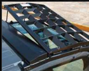
Standard FOPS overhead cab guard
